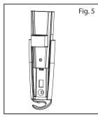
**IMPORTANT!** The set screw should be used at all times to prevent the mount from moving or rattling.
